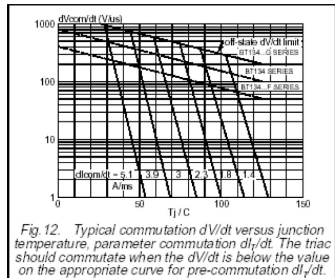
Fig. 12. Typical commutation  $dV/dt$  versus junction temperature, parameter commutation  $dl/dt$ . The triac should commutate when the  $dV/dt$  is below the value on the appropriate curve for pre-commutation  $dl/dt$ .
