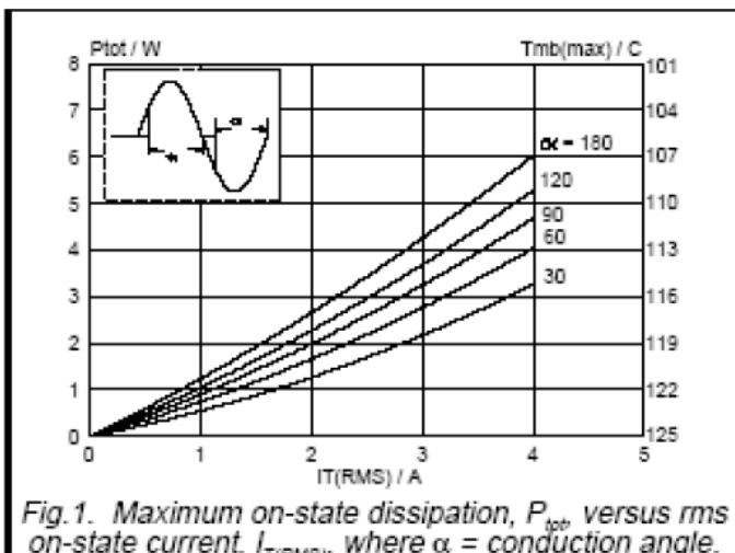
Fig.1. Maximum on-state dissipation,  $P_d(\text{on})$ , versus rms on-state current,  $I_{T(\text{RMS})}$ , where  $\alpha$  = conduction angle.
