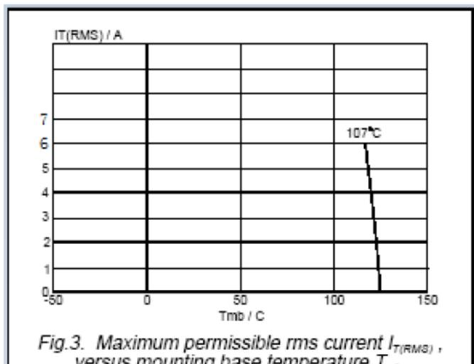
Fig.3. Maximum permissible rms current  $I_{T(\text{RMS})}$ , versus mounting base temperature  $T_{mb}$ .
