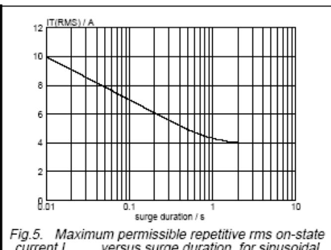
Fig.5. Maximum permissible repetitive rms on-state current  $I_{T(\text{RMS})}$ , versus surge duration, for sinusoidal currents,  $f = 50\text{ Hz}$ ;  $T_{mb} \leq 107^\circ\text{C}$ .
